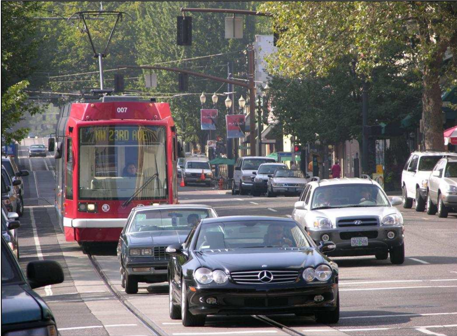
Most North American Streetcar systems operate with smaller, lower capacity vehicles that run in traffic with little or no priority (Portland, OR).
