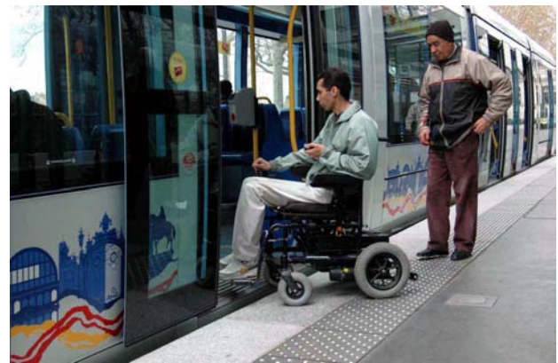
European Street Trams are modern, low floor (level boarding) and fully accessible (Lyon, France)
